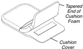
FIGURE 2 - REMOVING/INSTALLING LATERAL SUPPORT CUSHION FOAM
